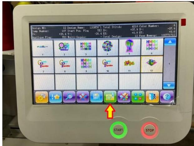
3. Scroll down to the color change that you want the machine to stop at prior to continuing the design using the arrows on the screen
